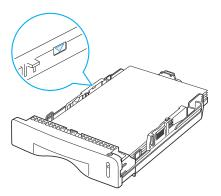
6 Insert and slide the paper tray back into the machine.
